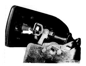
**Note:** The clearance between driving pin and counterpart on door lock should amount to approx. 1 mm. Adjustment is made at hex. screw (arrow).
