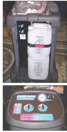
Robinair's new 75700 CoolTech, which uses a push/pull process (pressure at inlet, venturi vacuum draw), has two new-coolant tanks stacked in the back. The machine, which comes with adapters for connection in series with the radiator and upper hose, also can perform reverse-flushing with the engine off. The machine's top-mounted control panel has just two manual valves, for simplified operation.
