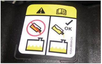
This pictorial label on a Ford vehicle (above) has a diagonal line through the orange, which means do not use orange coolant (really referring to DexCool). The "OK" refers to the use of yellow coolant in this cooling system.
