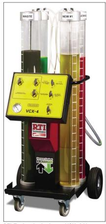
RTI Technologies' new VCX-4 Vacuum Coolant Exchanger comes with four coolant cylinders—one for used coolant and three for new coolants (such as DexCool, G-05 and conventional American). This machine, which uses shop air and venturi vacuum to do the job, is designed to connect to the radiator neck.
