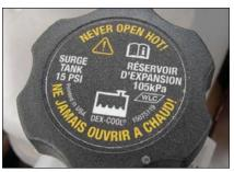
This Saturn cap reads DexCool, and that's what's inside, despite engine supplier Honda's objections.
