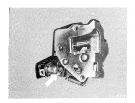
Note: The clearance between drive bolt and counterpiece on door lock should amount to approx. 1 mm. Adjustments are made on hex. socket screw (arrow).
