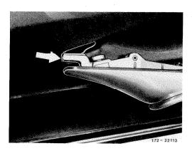
6 Introduce door handle at the rear, while turning key for approx. 50  $^{\circ}$  to the rear and introduce pivot rod into pivot nut on lock.
