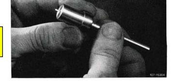
8 Clean nozzle needle with a sharp-edged hardwood stick soaked in diesel fuel. If profile of nozzle needle is badly coked, needle maybe clamped for this purpose in a suitable chuck of a lathe or drilling machine at its pressure pin (13). The spray pintle (8), the throttle pin (9) and the needle seat (10) can be cleaned with a sharp-edged hardwood stick soaked in oil.
