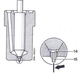
5 Buzzing test. Push hand lever slowly fully down (approx. 1 stroke per second); a damped buzzing of injection nozzle should be heard.
