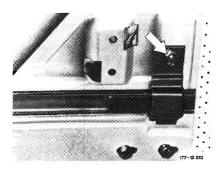
4 After opening the sun roof lid halfway loosen the left and right stop rod screws and adjust, so that the sun roof lid can be stopped in any position and the end lever can be operated with normal force. Also make sure that the sun roof is in the center of the opening.
