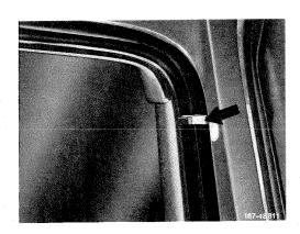
5 Expose copper wire in adhesive cord and make bright at ends with emery paper.
