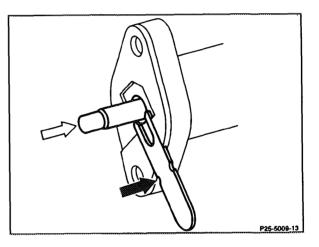
If notches are visible: Wear limit of disk has been reached.
