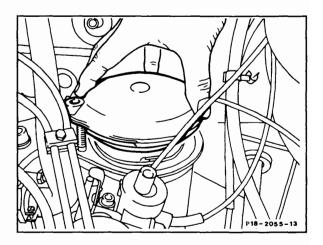
Suction engine oil via oil dipstick tube with engine at operating temperature.
