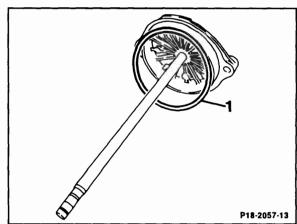
Check the oil port on the oil tube for foreign matter (arrow). If it is blocked, remove the foreign matter by hand. Then blow through the oil port with compressed air; air must noticeably come out of the bottom of the oil tube. If the oil port is not open or if no air comes out, replace oil filter cap and oil tube.
