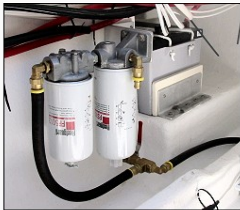
Simple and effective Multi-Stage Fuel Filter System. No messy & leaky bowls to deal with...
