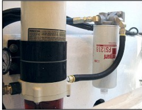
Racor 1000 w/ HD FS1218 Fleetguard primary bulk separator - Good for 700 hp
