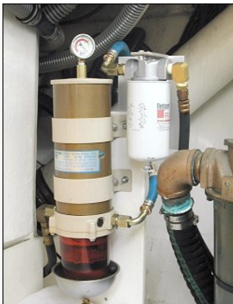
Simple and very effective upgrade for Racor's - Adding a bulk separator as the primary
