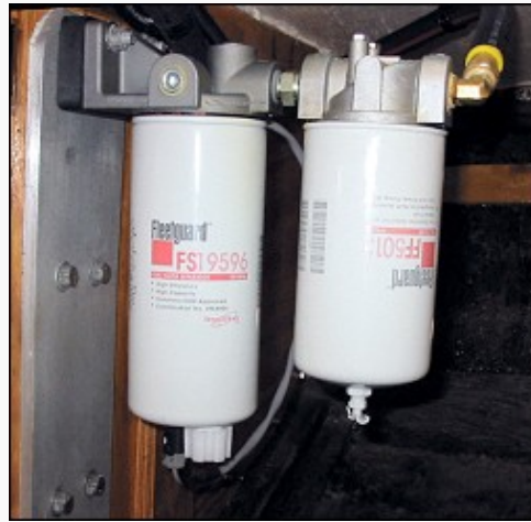
Basic Common Rail Fuel Multi-Stage system with WIF sensor - 100% Cummins, 100% simple, and 100% effective
