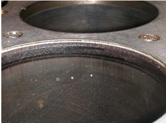
This is a slipped liner
