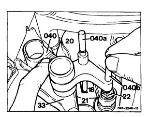
Slip long pin against backing plate of inner pad and short pin against head of caliper to brake carrier mounting bolt.
