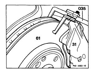
**Note:** Wear limits for brake disks must be strictly observed.
