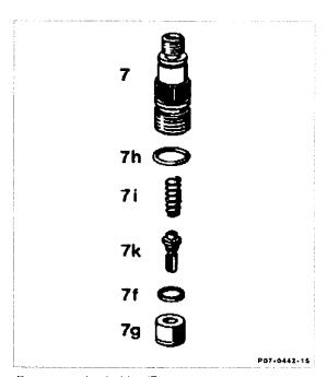
Pressure valve holder (7) tightening torque 35 Nm, special tool 617 589 01 09 00.
