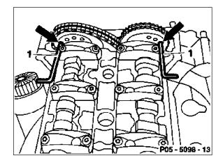
6 Rotate crankshaft back **in opposite direction** of rotation of engine to TDC position (arrow) with wrench 001 589 65 09 00.
