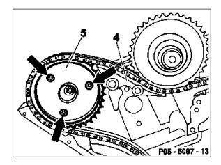
5 Rotate camshafts with wrench 104 589 01 01 00 until the 4 mm holes in the camshaft flanges (arrows) are at the top edge of the cylinder edge.
