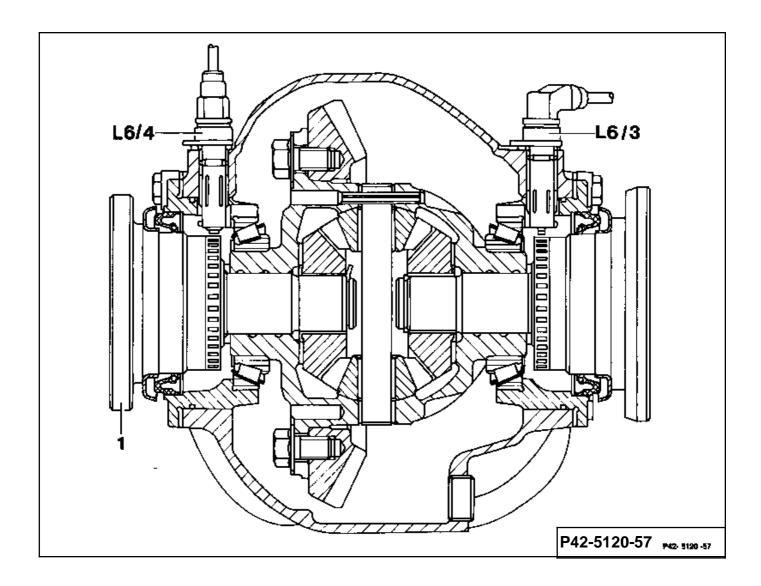
L6/3 Left rear axle speed sensorRear axle shaft flange with serrations
