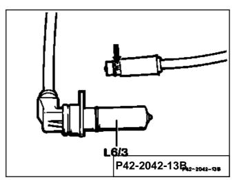
Right rear axle speed sensor (L6/4) is identified with "D" on the plug (arrow).
