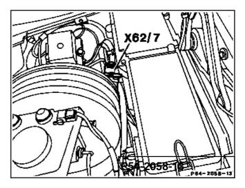
Location of the plug connection, left front axle distributor (X62/7) in left of the front axle component compartment.
