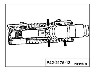
2 grooves (arrows) are cast on the side of the ASR control unit at the guide for the connector. On the right of the locking device is a web at various positions (arrows). The control unit comprises various circuit boards which are equipped with electronic components.
