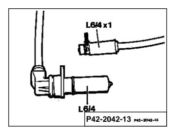
The plugs (D, E) of the left or right rear axle speed sensors (L6/3 or L6/4) are plugged into the plug connection, rear axle distributor (X62/8) into the openings marked "D" and "E".
