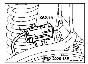
Location of the plug connection, left front axle distributor (X62/14) on steering knuckle.
