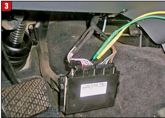
Testing N2 and N3 speed sensors in reference to battery ground
