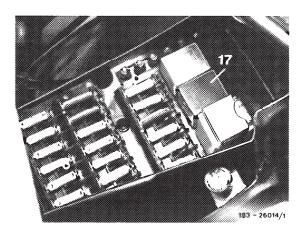
Location of relay (17) for auxiliary fan via pre-resistor (18)
