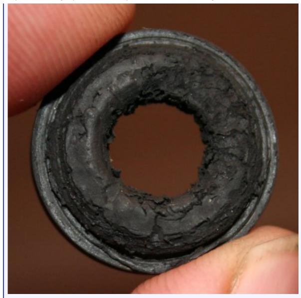
There are two more identical seals in the lower half of the valve. Take a screwdriver, inserted through the lower hole and press against each of the two seals and the brown plastic retaining cylinders. A little bit of force is needed to dislodge them. Once free, you can pull them out by hand and then pry out the rubber seals.
