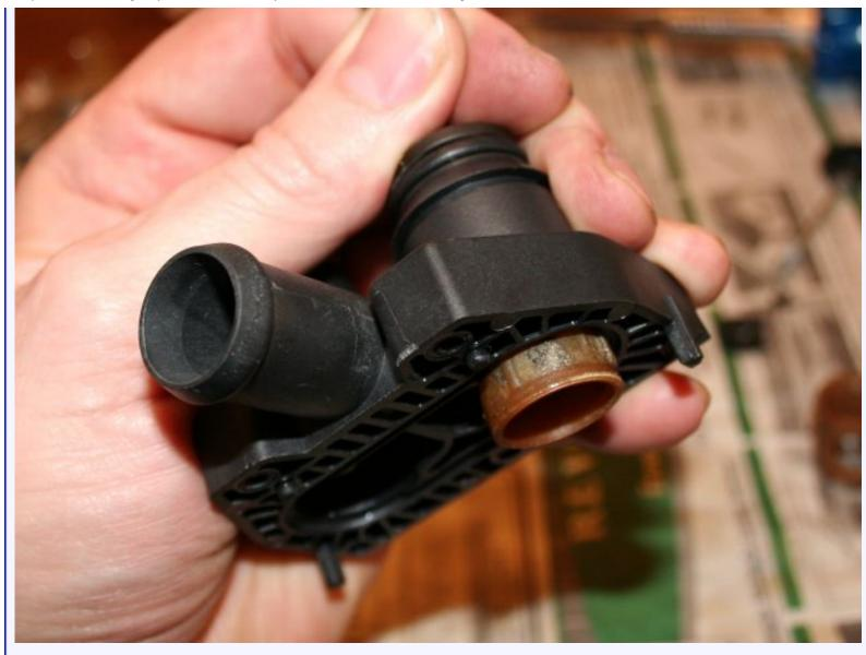
There will also be 2 O-ring seals, one between each section. Depending on the condition of the parts, you may need to do some trimming to make them usable again. I took a pair of scissors and carefully trimmed the excess rubber of in order to re-use them. The two pieces on the right were discarded.
