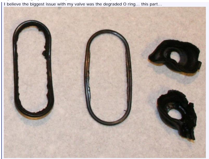
The center section from that seal was all gummed up inside the valve. Probably would have had a pretty good chance of the valve working right just by cleaning up/trimming the center section as outlined in the instructions (and also removing the tattered bits, of course). I was able to scavenge a similar seal off the surplus E320 valve I found.
