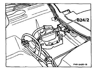
The ABS control unit (N30) processes the signals from the lateral-acceleration sensor (B24/2) and transmits control signals to the switchover valve in the master cylinder (Y61). Operating voltage is supplied by the basic module (N16/1). The control units are installed in the module box.
