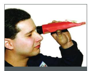
A refractometer provides the most consistently accurate indicator of freeze protection of a coolant mixture, and should be used by a professional technician, instead of a hydrometer or test strip.
