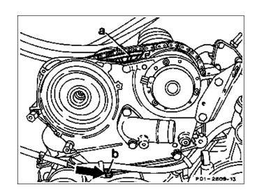
3 Engine 104.98: unbolt heating water return pipe (25) from the fan bearing bracket (28). Unbolt guide pulley (32).
