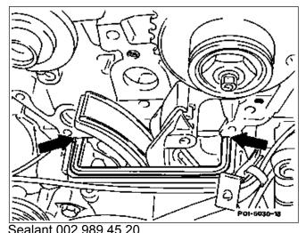
New shaped rubber gasket (24) insert dry (without sealant) into the oil-free
