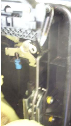
On my car the green rod should be held in the blue hole by a plastic bush. This was my problem. Also bruit force had been used in the past and the lever mechanism was damaged.
