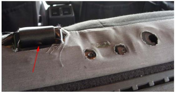
The red wire will need to be pulled up to release the centre hinge lock together with the side lock release, thought I was able to release the two locks one at a time. This wire can I believe also be the cause of a stuck seat, if it brakes or the adjustment unscrews itself.
