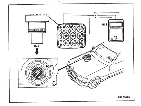
Fault table, DTC readout, Diagnostic module (N59)
