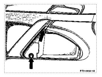
7 Press door liner off of interior door panel at bottom, front and rear with plastic wedge 110 589 03 59 00 (9 clips); insert plastic wedge directly at clip.
