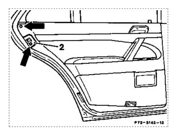
3 Unhook wooden cover at rear using special tool 140 589 16 63 00 by inserting blade of special tool between wooden cover and upholstery on door panelling, then pull special tool all the way up.
