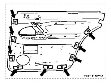
18 Install cover plate on door lock and screw down. Screw in screw on door liner (arrows).
