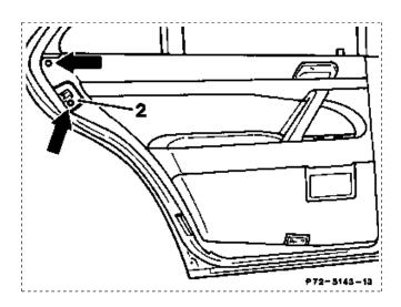
19 Install wooden cover; turn both catches to installed position.
