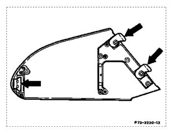
20 Insert wooden cover with catches into recess in door covering.
