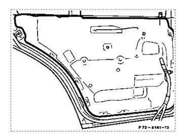
13 Complete electrical connections on door liner, guide wires through liner.
