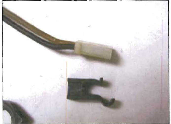
STEP 2: Pull plastic wrap back, remove clip
