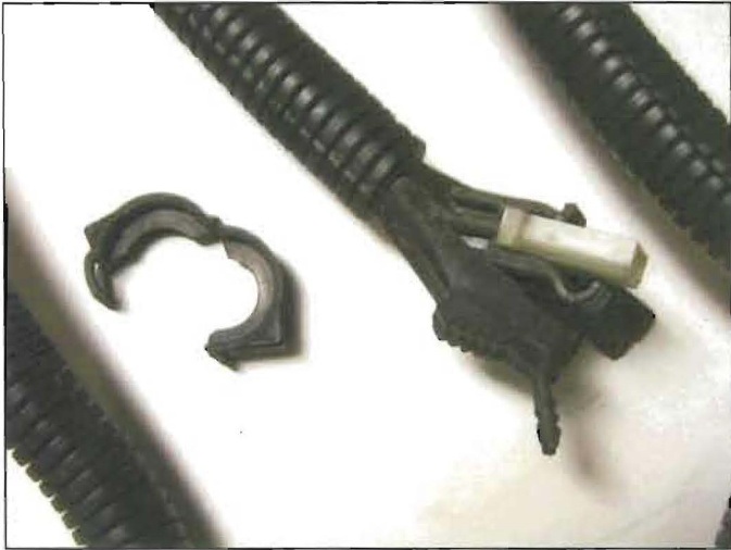
STEP 1: Remove snap ring from harness
