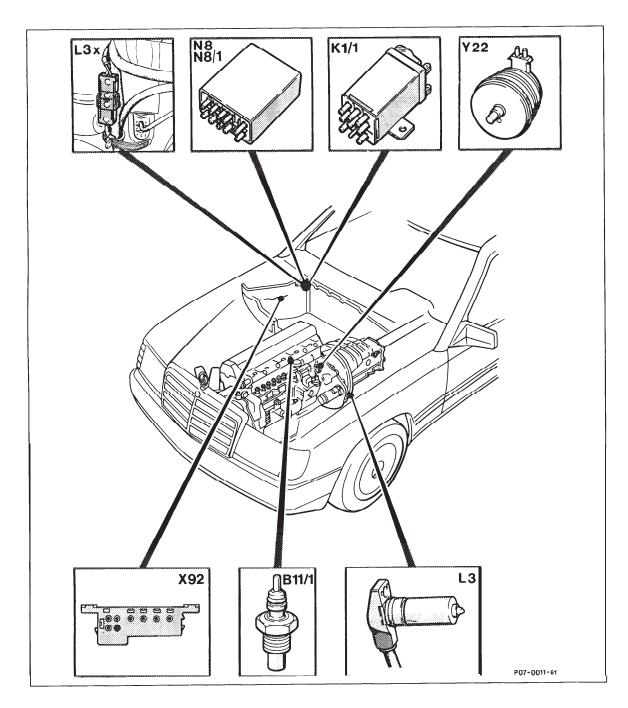
B11/1 Coolant temperature sensor K1/1 Overvoltage protection relay L3 Speed sensor
