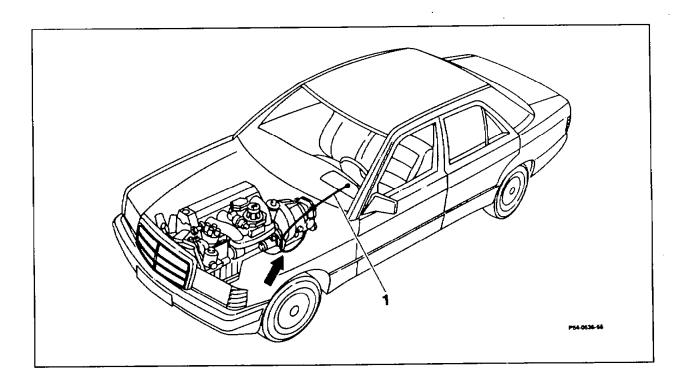
Speedometer shaft (1) at holder (arrow) ...... unclip, clip in. Carpet in left footwell ..... remove, insert. Speedometer shaft (1) from interior ...... push through downward, introduce from below.
