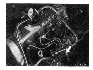
If final feed pressure is inadequate, exchange suction and delivery valves or fuel pump (07.1-235).
