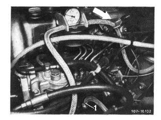
Measure vacuum pressure at idle speed. To do so, use clip to nip hose (arrow) at tester downstream of pressure gage.
