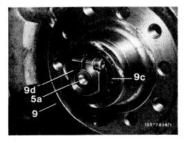
6 Place tester (015) on front wheel hub and set dial gauge (022) to approx. 2 mm preload.
