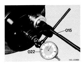
7 Check end play of wheel hub by energetic pulling and pushing at flange.
