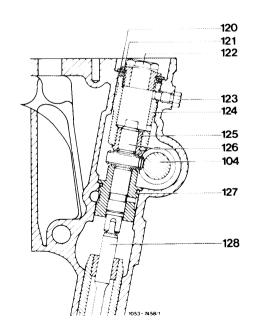
The O-ring seal (120) for the thrust piece is no longer fitted beneath cap (121). It is now inserted in a groove in the outside diameter of the thrust piece. Cap (121) has been discarded.
