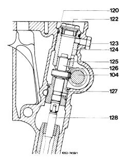
Owing to the modification of screw plug (122) from M 26  $\times$  1.5 to M 22  $\times$  1.5 it is necessary to use an adapter (part No. 616 589 00 63 00) to connect a mechanical rev counter.
