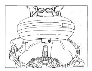
2 Check projection (K) towards torque converter housing.
