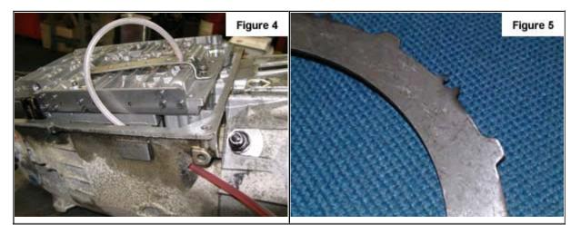
A steady stream of fluid would prove that the TCC piston was being hydraulically applied by cross leak oil. No steady stream of oil flowed out of the hose, so the test did not prove what was expected, but one very important piece of information was learned.
