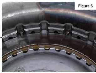
Ten springs were then added to serve as piston return springs (**Figure 6**) and Taa – Daaaaaa THE VEHICLE WORKED PERFECTLY!
