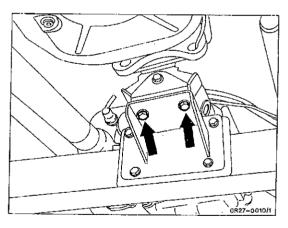
7 Mount universal-joint drive shaft and tighten to 35 Nm.
