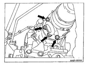
6 Unscrew twelve-point collar nut (14) and remove flange (13)
