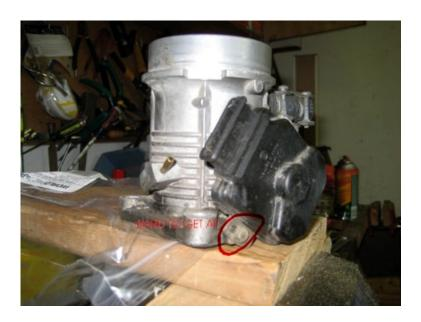
The throttle housing is easy to get off. Just 4 nuts and 1 hose. Don't drop the nuts – they disappear down into the Vee. But at least not into intake! That rag is important!
