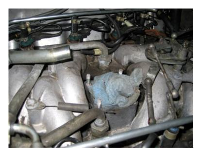
The TPS can just be pried off – It is held on by a spring clip. Once off, you need to get cover off. That plastic is old, but I found I could gently lever the tabs and then used a small screwdriver to release the cover:
