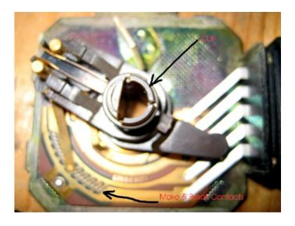
The shop manual shows which pins to use to check the switch. 12 & 17 test the idle switch. The resistance between these pins should be zero when the throttle is against it's stop. If the throttle is slightly opened (1 degree or 0.4mm feeler under stop), the resistance should go to infinity. This switch tells the ECU that you are idling.
