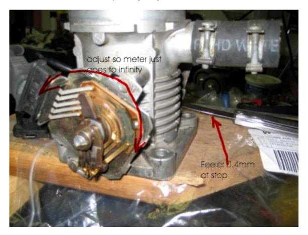
Once reinstalled, follow the instructions in the manual for linkage adjustment. Make sure the linkage is not preventing the spring from pulling the throttle lever against it's stop.
