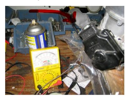
To adjust the idle switch, I placed a 0.4mm feeler gauge under the stop, then rotated the switch fully one way until meter read zero ohms, then turned slightly the opposite direction until meter read infinity. Clamped right there!
