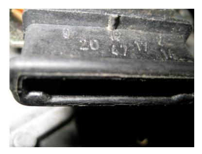
I found I could use a surplus injector plug to connect 12 & 20 for the idle test and 12 & 20 for the 10 step enrichment.
